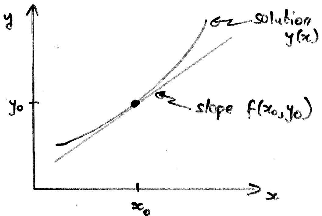
$f(x_0, y_0)$  determines slope of solution
